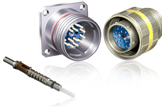
Figure 7. Glenair MIL-spec multi-fibre connector. 48-fibre versions are commercially available. It uses a modular design. The connector is built up of individual ceramic ferrule 'pin' inserts (shown in the picture below the connector halves).
