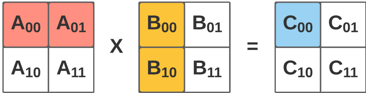
Figure 32: Blocked decomposition of the matrix multiplication of two 2 x 2 matrices. The entire AB product is decomposed into four matrix multiply operations (only the first is shown) operating on a 1 x 2 block of A and 2 x 1 block of B . C_{00} = A_{00}B_{00} + A_{01}B_{10} .
