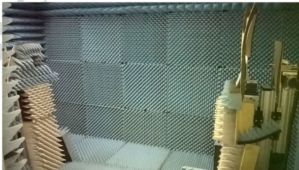
Fig. 3 Experimental setup for our laboratory tests at \nu = 20 GHz. The launcher (rectangular feedhorn) is visible to the left, surrounded by absorbing cones. On the right one can see the screen with the circular hole holding the TP and behind it the NF probe mounted on a linear stage to scan the field on an axis perpendicular to the direction of propagation, z . Later, the linear stage has been replaced with a two axis translation stage. All components are mounted on vertical supports that can be moved along z on an optical bench set on the ground, which is covered with absorbing panels in this picture
