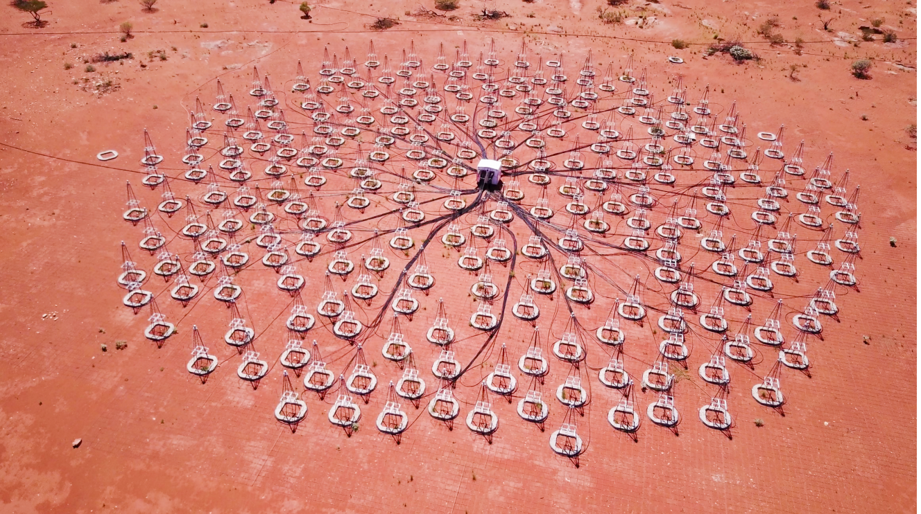
Fig. 11. AAVS1 in February 2018. The white box in the centre is the APIU, with the black hybrid cables running from each antenna to the APIU.
