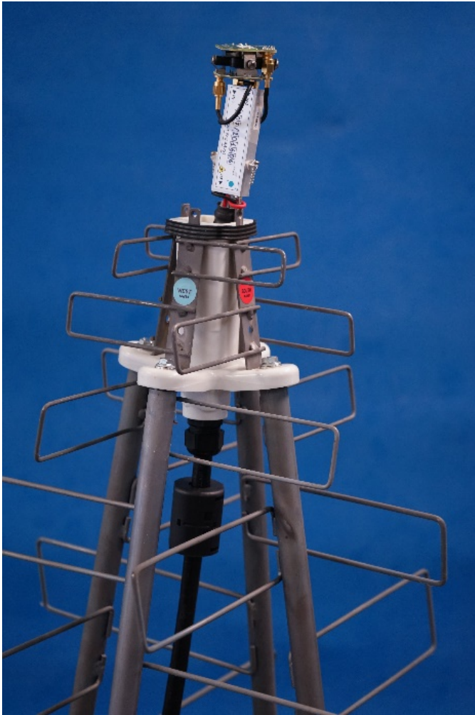
Fig. 5. Antenna electronics showing the top of a SKALA2 and the contents of the trumpet, including LNAs and the FEM. The hybrid cable runs down the centre of the antenna.
