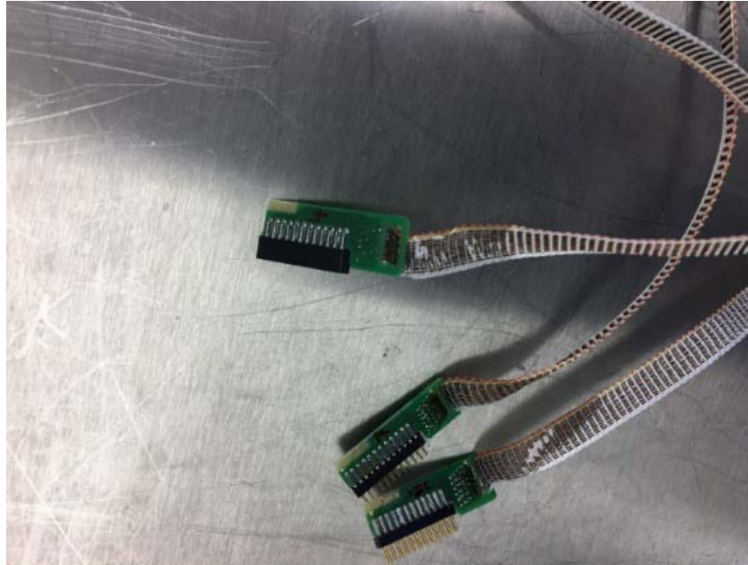
Fig. 5.5.2.2: example of a loom including its loom PCB
