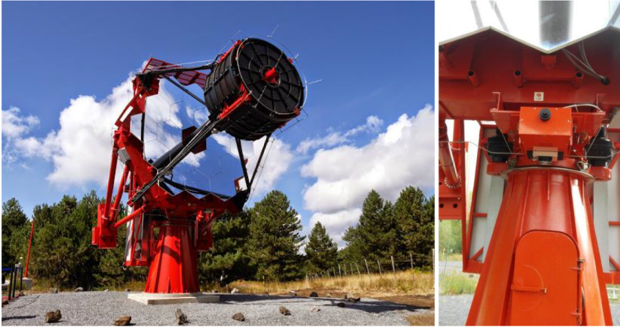
Fig. 1 ASTRI-Horn, the dual-mirror Cherenkov telescope installed on Mt.Etna, Italy, at the INAF “M.C. Fracastoro” observing station. On the right panel it is visible the small UVscope instrument mounted under the primary mirror structure of the ASTRI-Horn telescope
