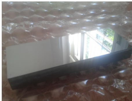
Figure 6: the beam expander crystal for the 4.51 keV setup, monocrystalline silicon, with the proper asymmetric cut at 44.59 deg from the (220) planes. The surface has been polished to remove the lattice damage introduced by the cut. The crystal dimensions are 170 mm x 60 mm x 20 mm
