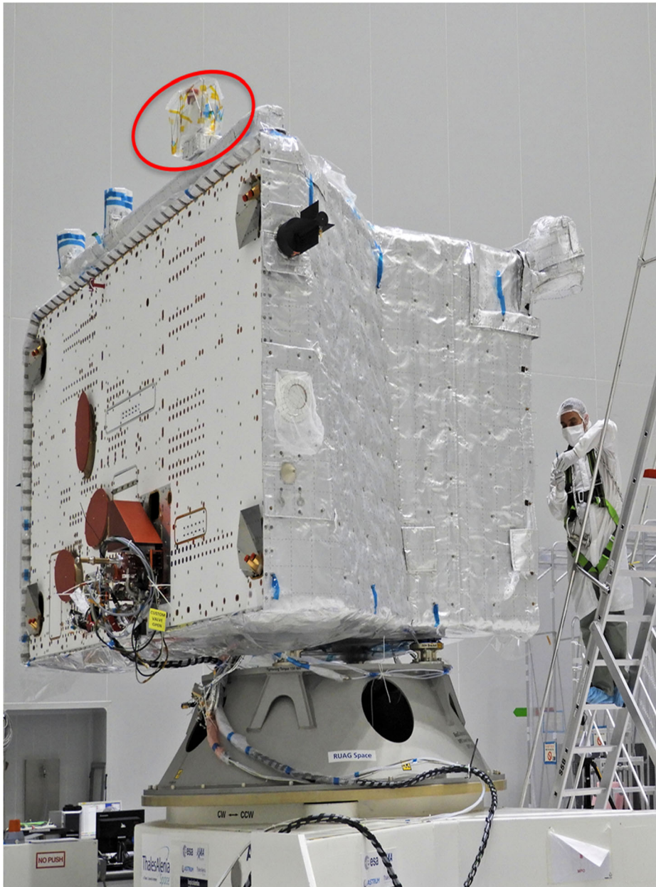
Fig. 4 SIXS sensor unit (in red circle) on the MPO spacecraft view from the radiator side. Photo courtesy of European Space Agency, ESA
