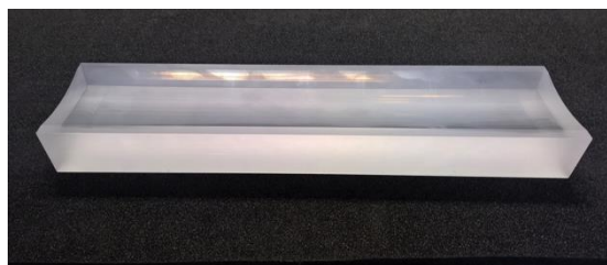
Figure 5: One of the two paraboloidal mirror in fused quartz HOQ 310, procured from Zeiss
