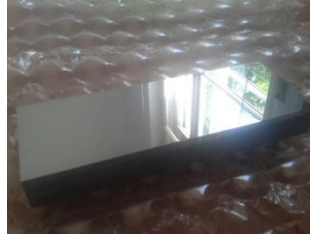
Figure 8: The beam expander in silicon for the 4.51 keV beam line. The surface has been polished to remove the lattice damage introduced by the cut (process done at CNR-IMEM). The crystal dimensions are 170 mm \times 60 mm \times 20 mm
