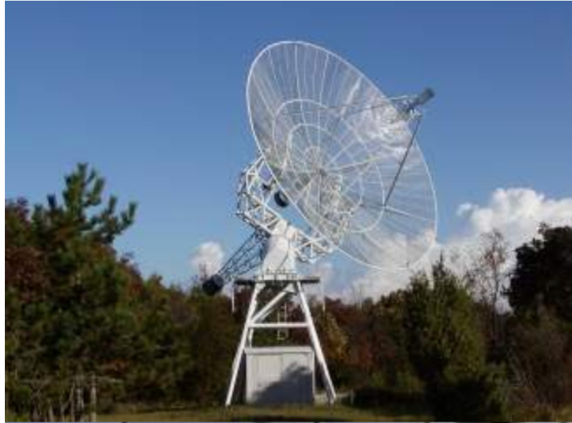
Figure 1. Metric Multichannel Solar Radio Polarimeter: a multichannel radiopolarimeter with 4 receiving channels in the band 200-800 MHz (237, 327, 408, 610 MHz), 10 m parabolic reflector with equatorial mounting.
