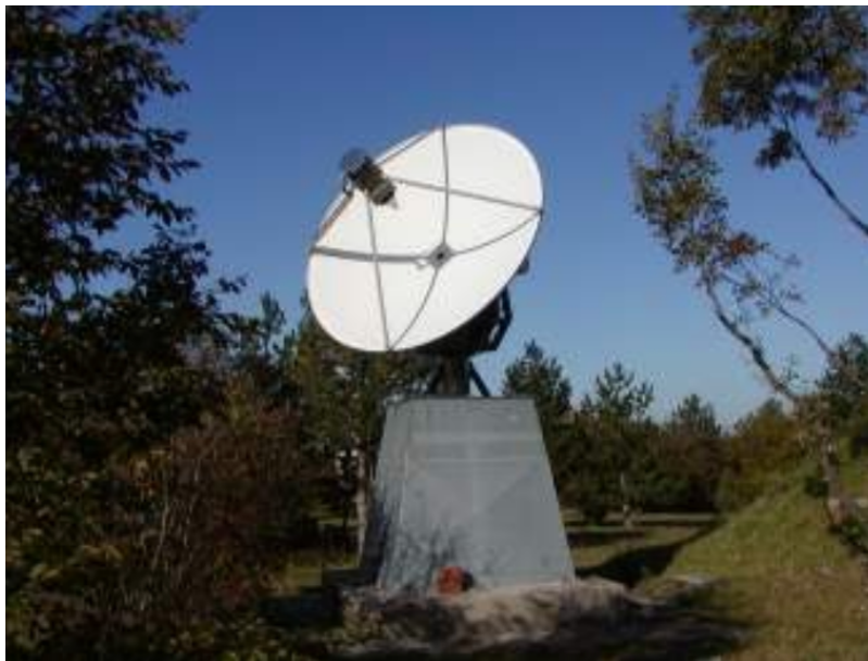
Figure 2. Decimetric Multichannel Solar Radio Polarimeter with 2 receiving channels in the band 1-4 GHz (1420 and 2695 MHz), 3 m parabolic reflector with alt-az mounting.
