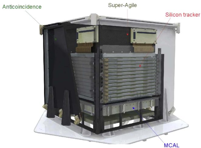
Figure 1. Sketch of the AGILE payload, not to scale. The main components are shown: the plastic scintillator Anticoincidence, the silicon–tungsten tracker, the CsI bars Mini-Calorimeter, the hard X-ray imager Super-Agile based on a silicon detector plane, and a tungsten mask.
