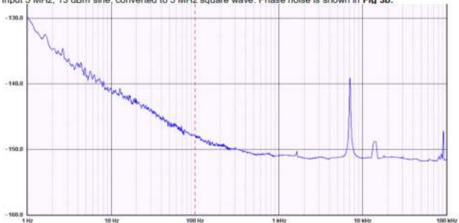
Fig 3b: Phase noise of 5 MHz square wave output, input 5 MHz sine input 13 dBm to input A.
