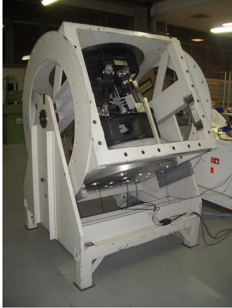
Fig. 2. The hexapod under test on a tilting device at ADS International srl premises (November, 2008).
