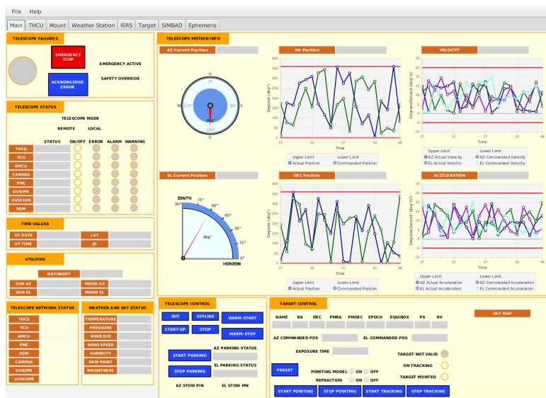
Figure 5: ASTRI Engineering GUI main view
