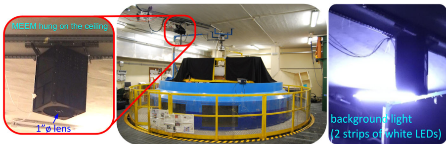
Fig. 3 The TurLab tank setup with the Mini-EUSO EM installed on the ceiling and enlarged inside the red frame (left). The diffused airglow in the atmosphere was reproduced by two strips of cold-white LEDs reflected by the ceiling above the tank (right)
