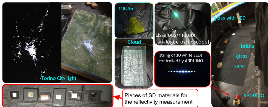
Fig. 4 Light sources and materials to reproduce phenomena that Mini-EUSO can observe. Reflections of materials that are often present in space debris (SD) have also been tested
