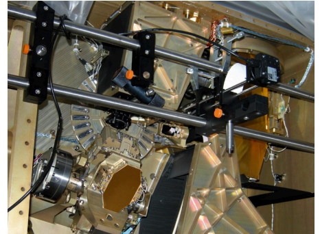
Figure 2. Close look at the VISIR low- and medium-resolution assembly. The unit in the lower left is the carousel, a precision rotary stage used to scan the gratings. At the top right is an optical bench with a CMOS camera rigged as proxy for the infrared optical axis. Slightly above the carousel the mount of the special prism can be seen, which compensates the alignment for the change in refractive index between the HeNe laser and the desired central wavelength ( 10.5\ \mu\text{m} ) and the thermal shift between room temperature and the operating temperature of VISIR ( \sim 28\ \text{K} ).
