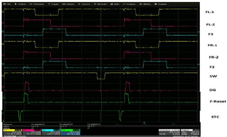
Figure 6. CCD horizontal phases and control timing.
