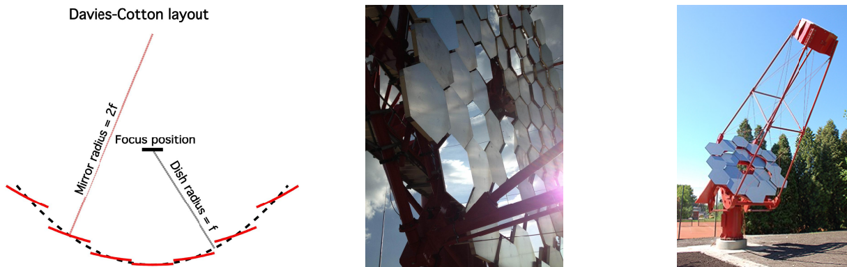
Figure 4 Left: Scheme of the Davies-Cotton optical design. Mirrors with radius of curvature 2f are arranged on a mechanical structure with radius f . Center: the MST prototype with the mirrors manufactured by the authors. Right: the SST-1M prototype with dummies.
