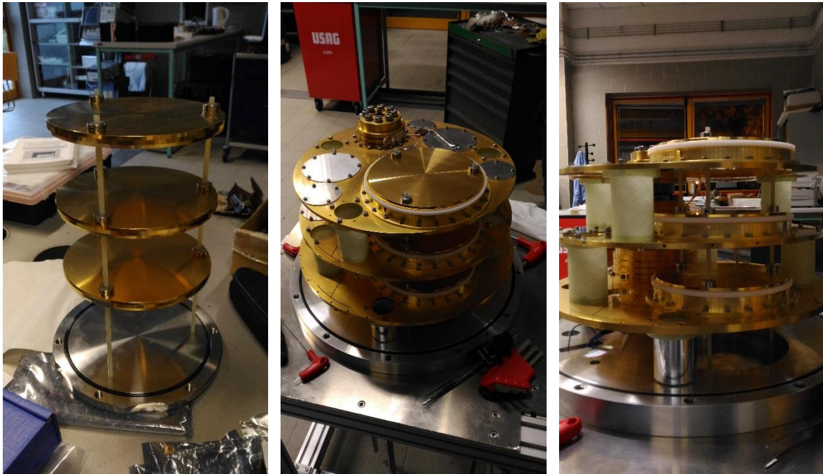
Figure 4 The dummy cartridge (left panel) which was integrated in the cryostat (middle and right panels) at its delivery to IASF Bologna and was cooled down during the first dry run
