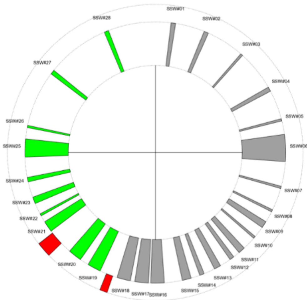
Fig. 7. DREAMS mission timeline for operation in day 1 showing sensor activation windows (in green) after expected landing and orbiter passage timelines (in red) in Mars local Time. (For interpretation of the references to colour in this figure legend, the reader is referred to the web version of this article.)
