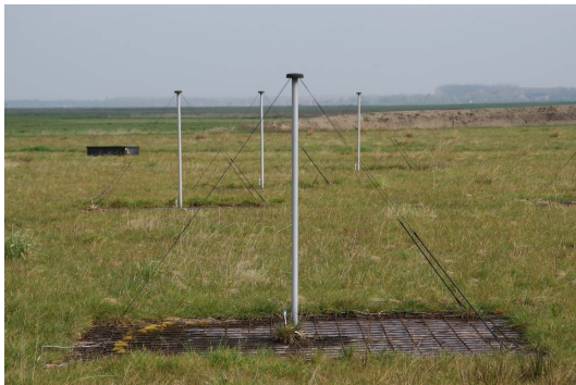
Fig. 3. Sensor of LOFAR LBA sub-array.
