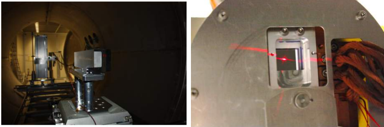
Figure 9: the BEaTriX mirror at PANTER. Left: before coating, in the PANTER vacuum tank. The detector stage, housing the TRoPIC and the PIXI detectors, is visible in the background. Right: the alignment laser, sharply focused on the TRoPIC sensor.
