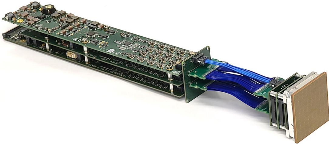
Figure 10: A single SST Camera Module, consisting of a 64-pixel SiPM tile, connected directly to PCBs providing SiPM bias voltage and signal preamplification. Flexible ribbon cables connect to the TARGET module, providing digitisation and first level triggering.
