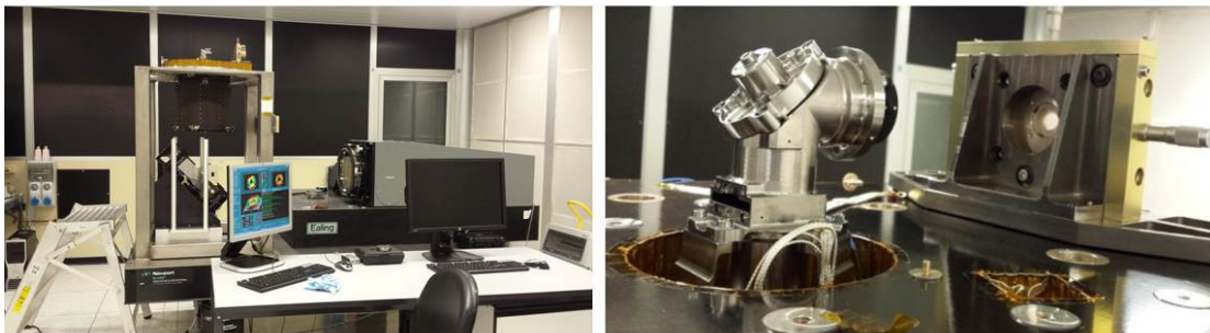
Figure 6. TEL in vertical position illuminated by the interferometer in double pass (Left). The reference spherical mirror mounted on the top of the optical bench (Right).
