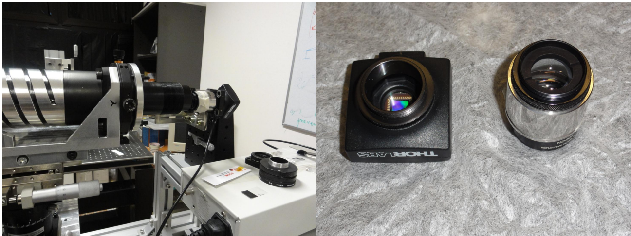
Figure 11 Measurement of the radiance uniformity in FC configuration; on the right, camera and objective used to measure the radiance uniformity.
