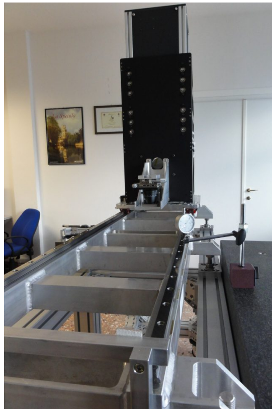
Figure 5 An adjustment of the vertical straightness deviations of the rails was carried out by means of repeated measurements at a distance of 60 mm and systematic insertion of shims. A 0.01 mm resolution dial indicator sliding on a 1 m long, DIN 876/0 class granite inspection table was used.
