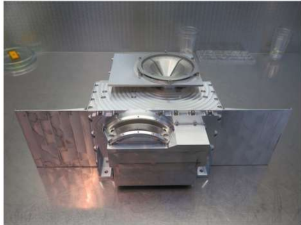
Fig. 23 The SCIENA fully operational Technology Model, excluding some thermal hardware
