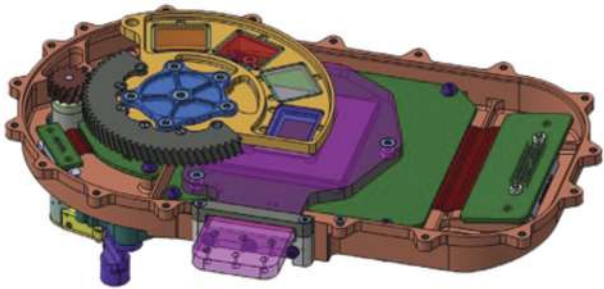
Fig. 17 The CoCa filter wheel assembly with four filters. The detector is shown in pink below one of the filters. The filter wheel includes a launch lock to prevent motion during launch
