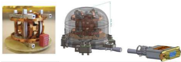
Fig. 30 Picture of its sensing elements (left) and CAD rendering (right) of one FGM-B2 sensor
