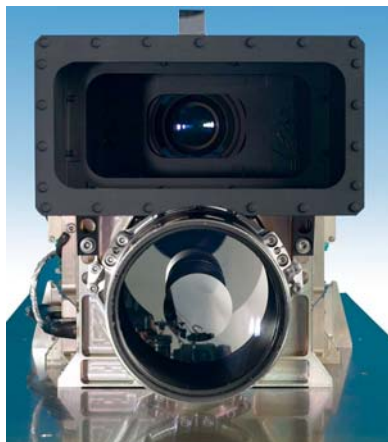
Fig. 1. Mars-Express HRSC camera optics (top: stereo camera optics, bottom: Maksutov-Cassegrain optics of the SRC)
