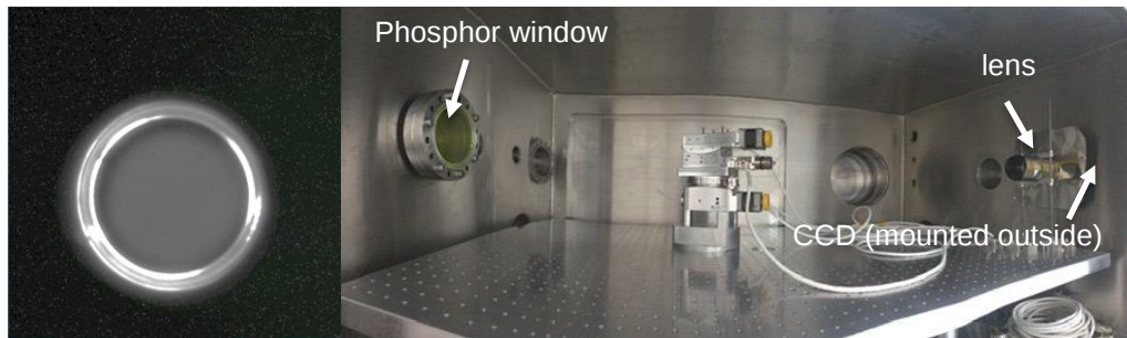
Figure 5. Monitoring setup inside the Optical chamber to align the X-ray source to the SA (right). Visible image of the X-ray source, created on the phosphor window (left): the bright rings are the light scattered from the edges of the window, the uniform central circle is the direct light from the X-ray source after alignment.
