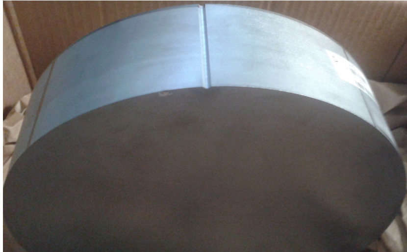
Fig. 11: the monocrystalline cylinder in silicon purchased from MEMC (20 cm diameter, 50 mm thick). The terminal surfaces are the planes (100). The lateral groove locates the (010) planes.
