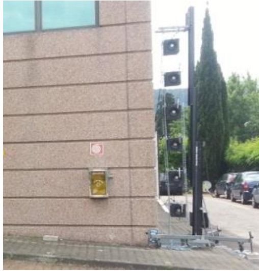
Figure 8 – Deployment of the ANC system at the corner of a building.
