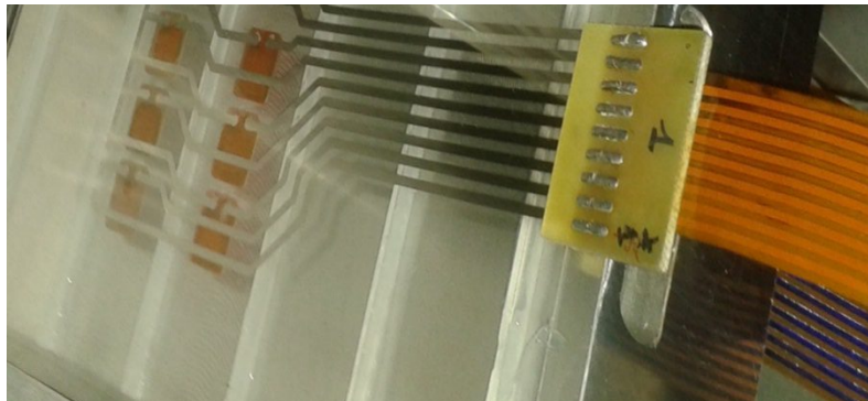
Figure 5. Ad-hoc connector and flex cable attached to the glass.
