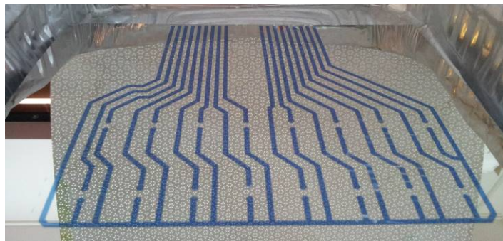
Figure 2. Electric tracks deposited on the back of a curved thin glass. They are still protected by a photoresist film.
