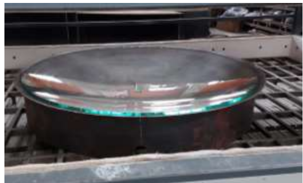
b) ASTRI M2 mould + slumped glass sheet
