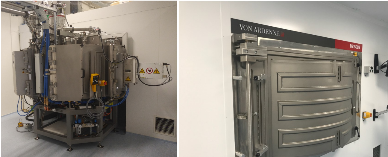
Figure 5 – Photographs of the newly installed drum coating machine for mass production of coated SPO plates. The left image shows the backside of the machine inside a grey room for easy access and service. The machine has a plasma cleaner, two magnetrons and space for a third one. The right image shows the front side of the vacuum chamber as seen from inside the cleanroom of cosine. The large door can be opened to load and unload carriers holding up to 150 SPO plates. The system is then closed, evacuated and the carousel moves the plates past the magnetrons to sputter single or multi-layers. The system is fully automated and the recipe can be set via the computer system shown in the right image.
