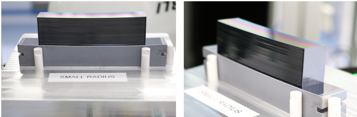
Figure 9 – Photographs of the very first 35 plate outer radius stack, produced in May 2018.
