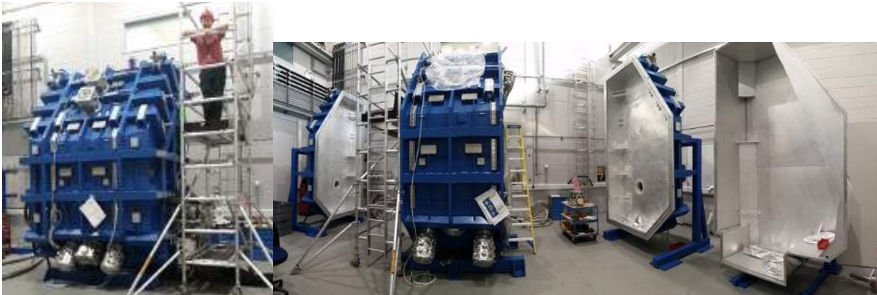
Figure 6. The MOONS cryostat (4.2 x 2.5 x 2.7 metres), on the left fully assembled, while on the right showing the two sections opened.
