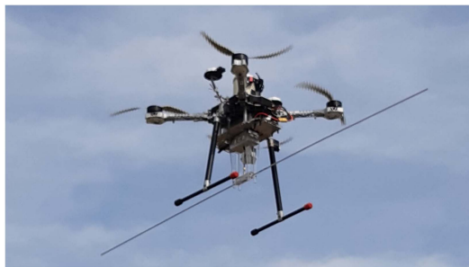
Fig. 3. UAV-mounted dipole hovering during the measurement.
