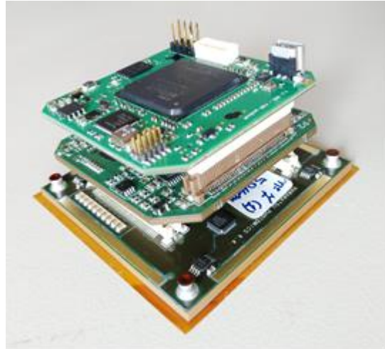
Figure 2. The stack architecture of the PDM (upside-down): from top to bottom, there is the FPGA board, then the ASIC board and then the SiPM board. The dimensions are 57.6mm x 57.6mm, with a depth of 30mm.
