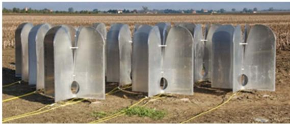
Figure 4: The Medicina Array Demonstrator with RF-over-fiber links (yellow cables).
