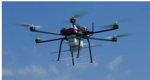
Figure 1: UAV-based flying test source. The payload consists of a GNSS receiver, an RF generator and a dipole antenna.
