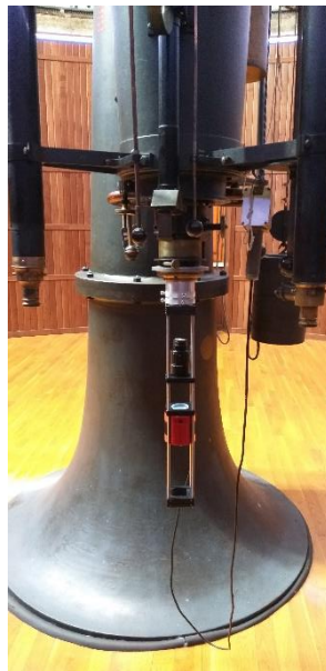
Figure 3. The CMOS camera mounted onto the telescope focal plane of the Cooke telescope for the acquisition of Mars' and Jupiter's images (an optical adapter is placed between the camera and the focal plane to test different magnifications).
