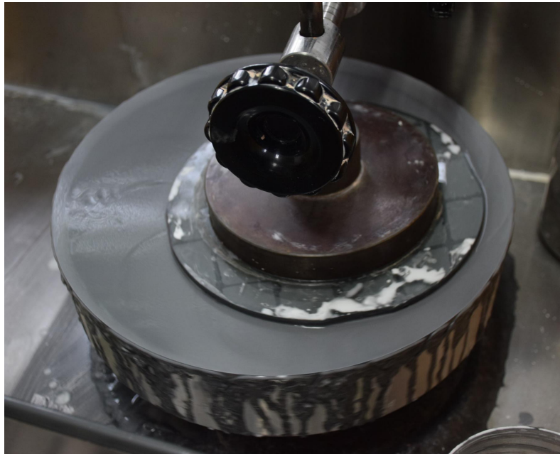
Figure 9. Grinding process for left surface of Lens 4. Note the glass tool over the workpiece.
