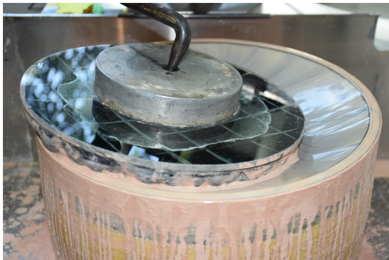
Figure 10. Polishing process. Note the pitch tool over the workpiece.
