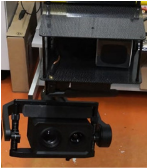
Fig. 2. Gimbal that hosts a HD VIS camera and an IR camera for night vision.
