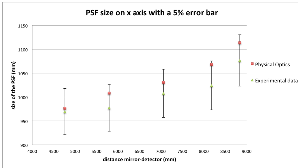
Figure 6. Comparison of the PSF size obtained using Physical Optics (red squares) and Experimental images (green triangles) for a mirror oriented at 8.79 deg from the source located at 8430 mm from the center of the mirror with a \pm 5\% error bar on experimental data
