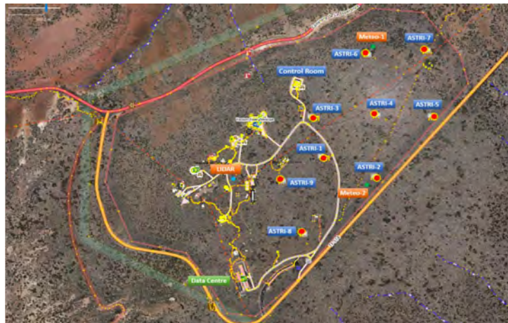
Figure 3: ASTRI Mini-Array general Layout The figure shows the final positions for the 9 telescopes, the roads to access each of them, the position of the two meteorological towers, the current position of the LIDAR, and that of the local control room (@Themis) and the data center (@Residencia). (Image obtained with Open Street Map editor).
