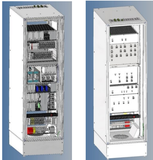
Figure 5. CAD model of the CUE. It hosts the CU control electronics, the optomechanical modules for the fiber and filters selection, visible and infrared light sources and redundant power supplies in a liquid-cooled environment. The interface panel for the connections (cable & fibers) with the CUMB is on the top side. The front side (left) allows the inspection of visual indicator lights and fast maintenance operations. Internal connector interfaces and power switches are placed on the rear side (right).
