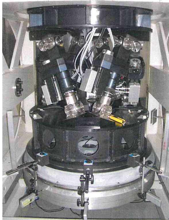
Fig. 1 – The VST hexapod connected to the astatic levers support system and to a metallic dummy of the mirror.
