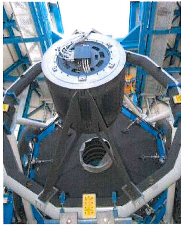
Fig. 7 – The secondary mirror support system integrated in the telescope in Chile.
