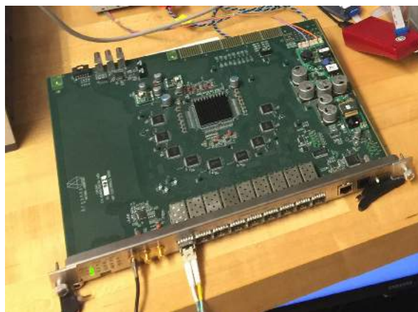
Fig. 36 Photo of the demonstrator DIAT on a laboratory test stand, connected to the pSCT camera backplane. The DIAT is a single-board custom-designed module for time-tagging, timing synchronization, hit pattern processing, and cross-triggering. Fiber optic ports on the front panel connect to up to nine SCT backplanes for the full-sized camera.
