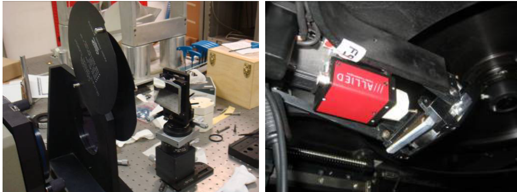
Figure 7 left side: the interferometric test of the pick-up mirror; right side: the pick-up mirror flexure test
