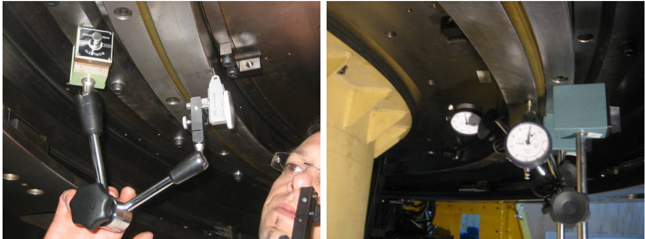
Figure 5: run-out (left side) and wobble (right side) test performed on the OMEGACAM bearing
