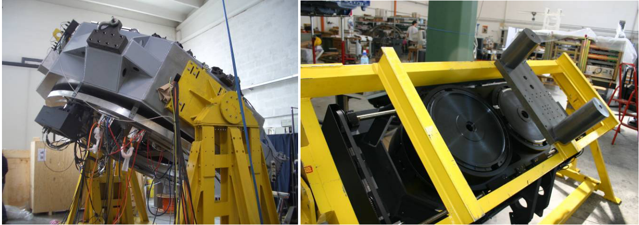
Figure 2: left side, the VST primary mirror cell mounted on the telescope simulator; right side, the ADC-Corrector system mounted on its handling device and tested at 45° altitude angle.
