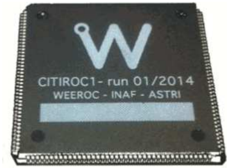
Figure 3: CITIROC chip 4.9 \times 4.6 \text{mm}^2 (courtesy of WEEROC).
