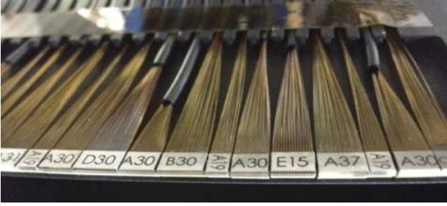
FIG. 7.— V-groove blocks aligned onto the SP1 pseudo-slit for the P-MaNGA prototype instrument. The V-groove blocks position the output end of the fibers that compose the IFUs and direct their light into the spectrographs.
