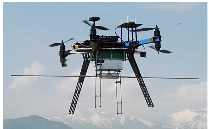
Fig. 1. The test-source consisting in a multicopter carrying a frequency synthesizer and a dipole antenna.
