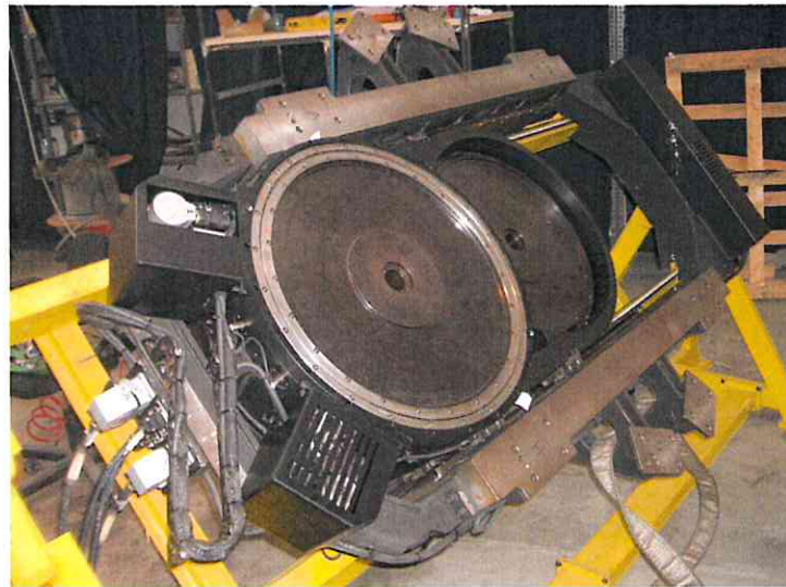
Fig. 7 – The ADC assembly installed on a tilting device to perform tests under realistic gravity conditions.
